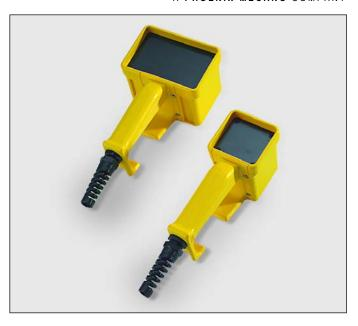
Control Units 2930 (left) and 2940: Each enclosure consists of a one-piece glass-filled polyamide enclosure body, polyester round-cornered front panel with screws, stamped foam rubber gasket, wall-mount bracket, and M20 cable grip. Power cord cable grips are designed to offer bending protection and strain relief.
